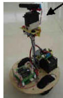
Figure 6. A Micro-Rato platform provided since 2003 and its beacon detector mounted on a servo (arrow).
