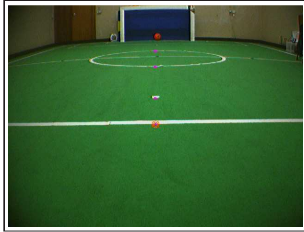
Figure 5.5: Example of an image processed by the tool PerspectiveMapCalib . Magenta spots in the image show the white lines found. Orange circles highlight the spot being processed.
