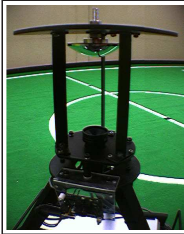
Figure 2.1: The hardware architecture of the vision system developed for the CAMBADA robotic soccer team. On the top, the omnidirectional sub-system with a camera pointing to an hyperbolic mirror. On the bottom of the image, the perspective sub-system with a camera pointing towards the field.
